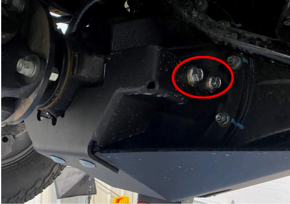
Figure 6 M10 Hex Bolt Correct Installation
