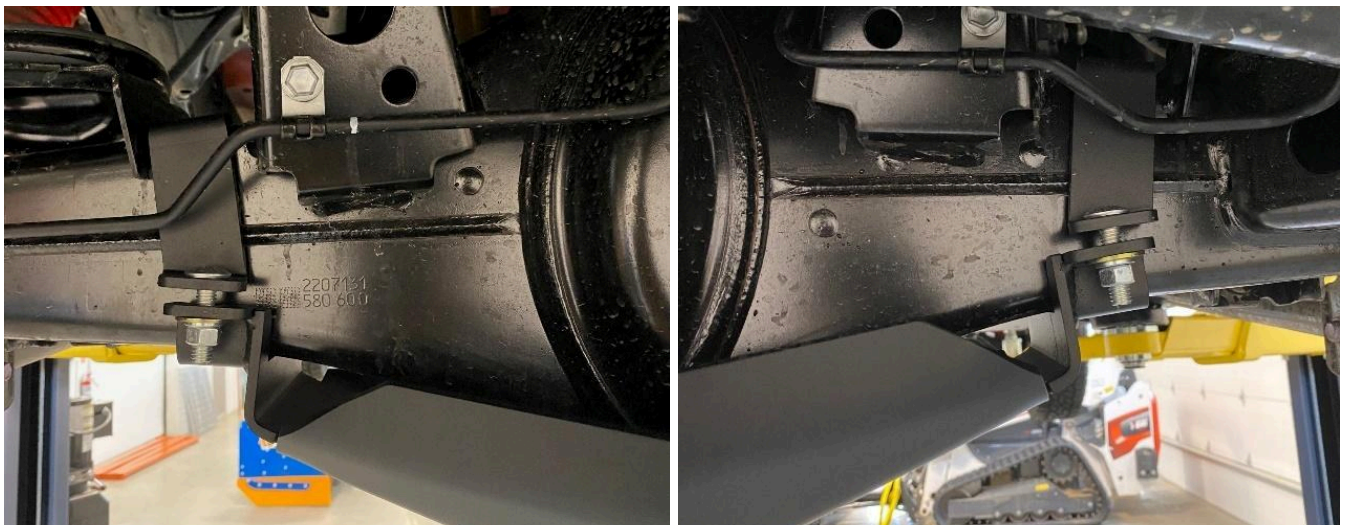
Figure 4 Rear View Top Axle Clamp Orientation
