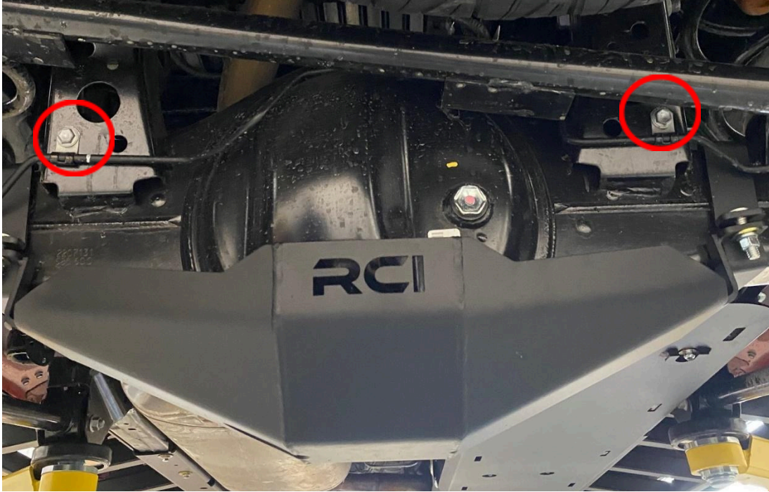
Figure 3 Brake Line Bolts to Loosen
