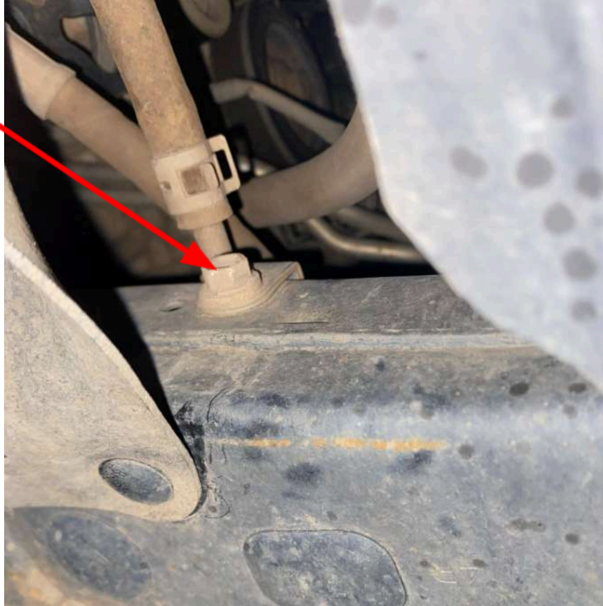
Figure 14: Mount located behind passenger wheel well splash guard.
