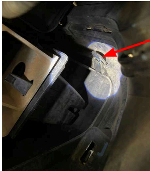
Figure 3: Image shows clips on back side of the OEM bumper
