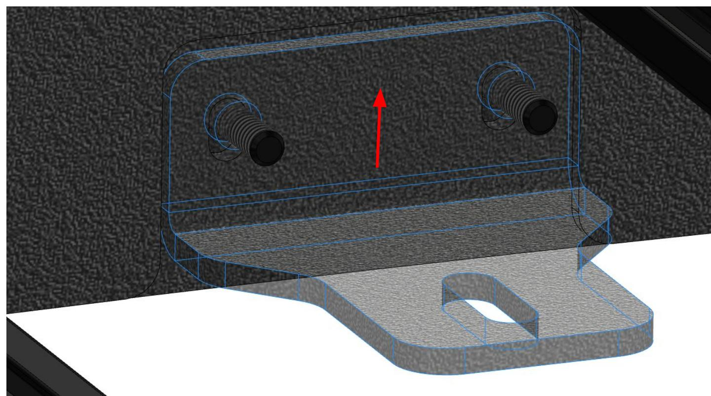
When bolting mounting feet to siderails, slide them to the highest position in the slots, this should give a  $\frac{3}{8}$ " gap between the side rail and the roof
