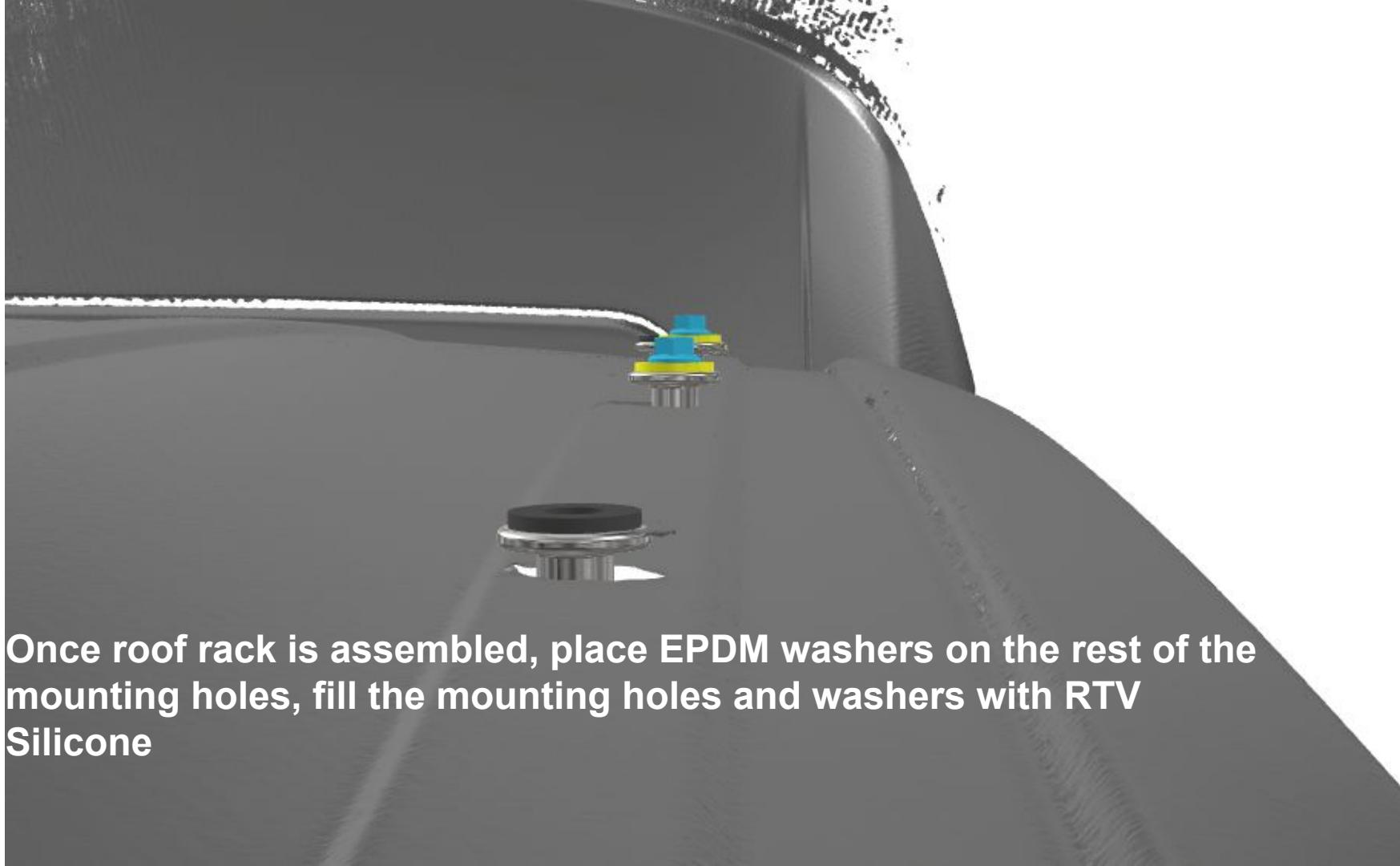
**Once roof rack is assembled, place EPDM washers on the rest of the mounting holes, fill the mounting holes and washers with RTV Silicone**
