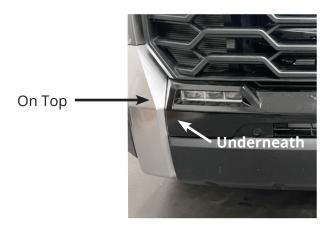
**Step 3:** With the fascia removed, uninstall the factory fog light using a Philips head screwdriver or carefully with a drill. Place the hardware in a safe location because it will be reused when installing the new fog lights. Now that the fog lights are removed, run the wire harness from the battery down to the fog light pockets. Make sure to zip the wiring away from any hot, sharp, or moving parts.
