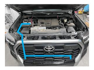
Connect the factory adapter plug to the factory fog light harness and then plug the blade terminal into the **GREEN** female spade connector. Leave the light bar plug accessible in the pocket. Route the other light bar plug over to the remaining side and leave it accessible. With the harness installed, connect the light bar to the harness and install the 6" light bar into the factory location using the factory hardware. Leave the hardware semi-loose to adjust the beam angle later in the install.
