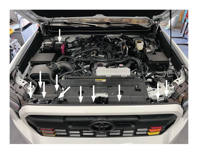
**Step 2:** Remove the fender flairs. The fenders can be removed by taking out two pins and 8 10mm screws, indicated with arrows. The fenders have plastic pressure clips that can be release by pulling the fender directly away from the body. The clips holding the air vent towards the front are very stiff and it may help to release the clip from inside the fender.
