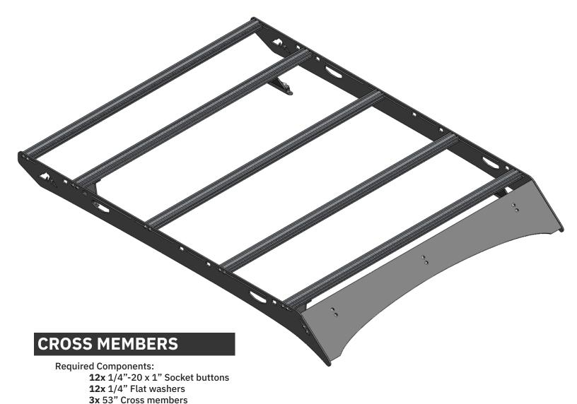
Secure all of the remaining cross members to the rack system using the 1" socket buttons and washers in the open slots in the sideplate. Position according to your load requirements.
