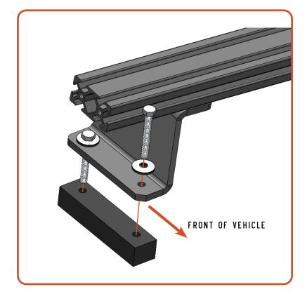
The bonded washers should compress and become flat, but not concave. Do not over tighten these mounts.
