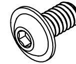
1/4-20 X 0.5 FLANGED BUTTON HEAD HEX DRIVE SCREW
