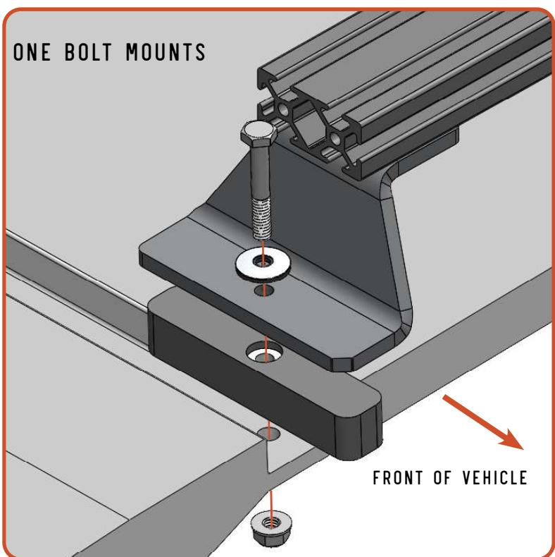
The bonded washers should compress and become flat, but not concave. Do not over tighten these mounts.
