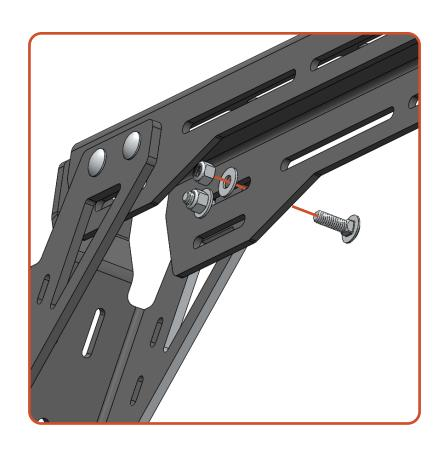
For flush installations, use the **top set of mounting slots**. For tents, use the **lower set of slots** to raise the crossbars by 1". (Does not apply to mid height towers)
