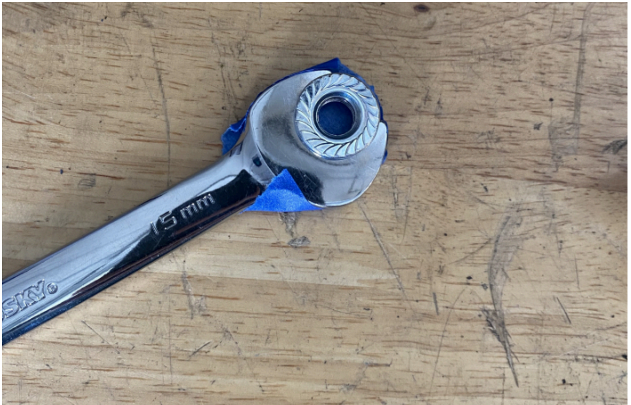
Figure 1: Tape M10 nut on 15mm wrench.
