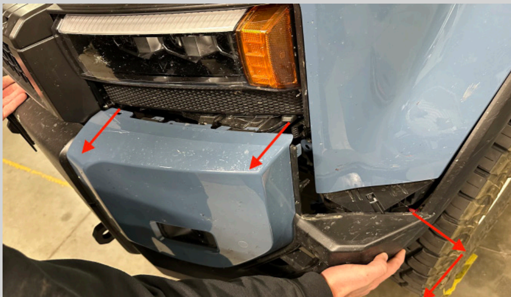
Figure 11: Removing the bumper cover.
