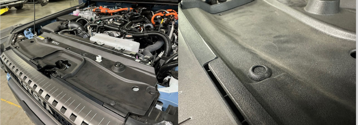
Figure 1: Left - Radiator cover to be removed. Right - Plastic clip depressed so it can be removed and the radiator cover removed.
