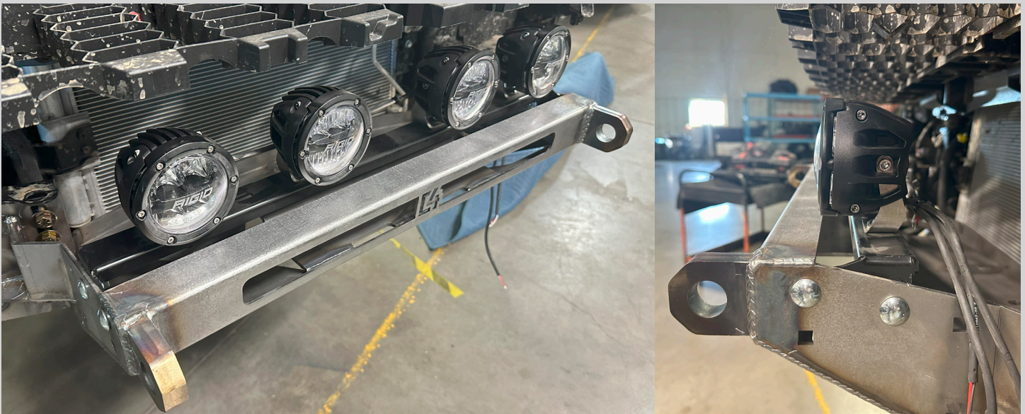
Figure 23: Grille light bracket mounted in the lo-pro.
