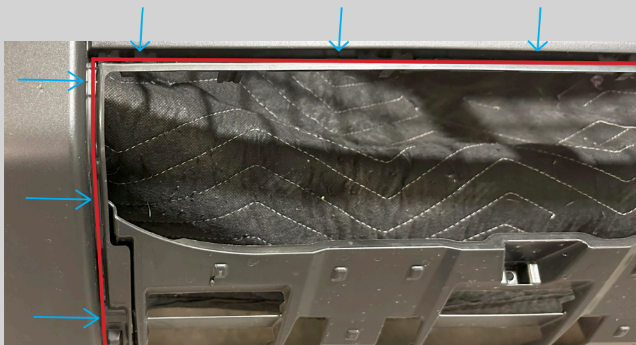
Figure 18: Make sure to cut in the corner along the sides and top of the bumper cover or down in the flat spot (red line) and sand the edge back to the molded edge of the bumper cover (blue arrows).
