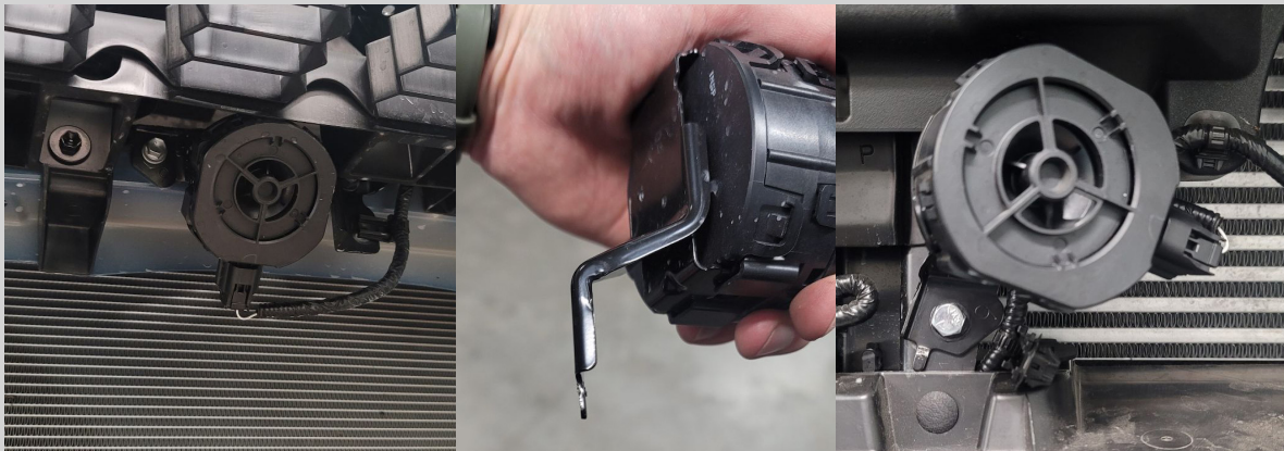
Figure 22: Keyless door lock “beeper” relocation.
