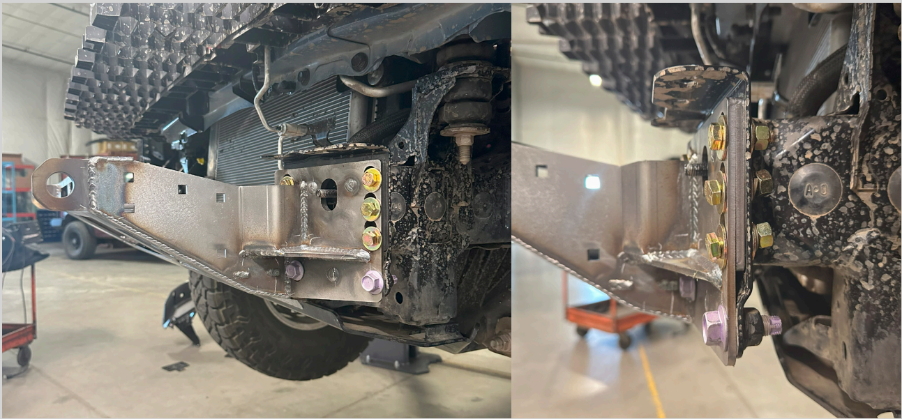
Figure 24: Hardware loosely installed, bumper raised to center of adjustment and top and bottom outside hardware snug.
