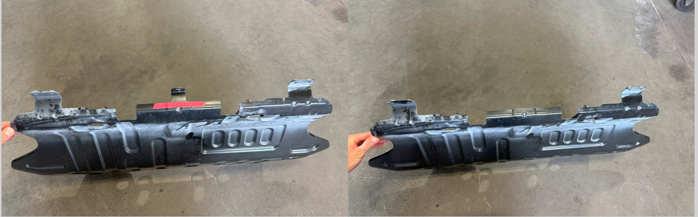
Figure 25: Mark and cut off the center tab on the skid plate.
