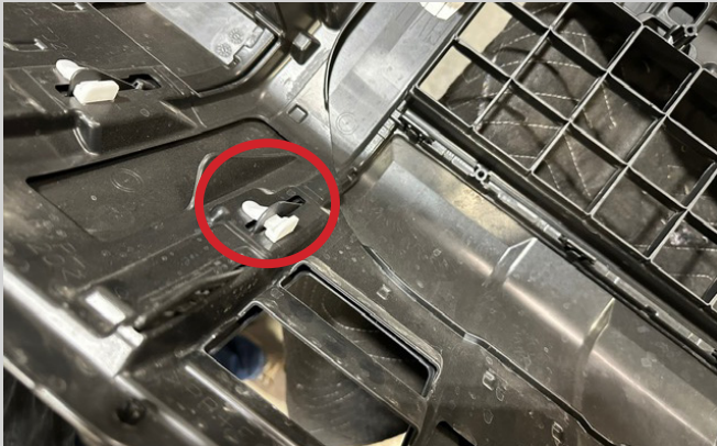
Figure 12: Remove the white clip on each side
