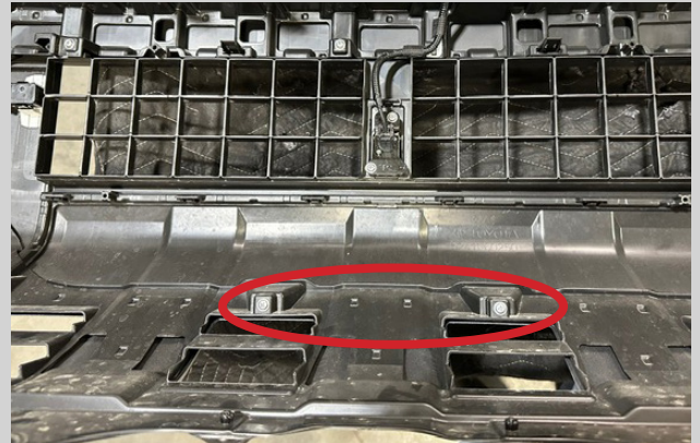
Figure 13: Remove the two screws in the center
