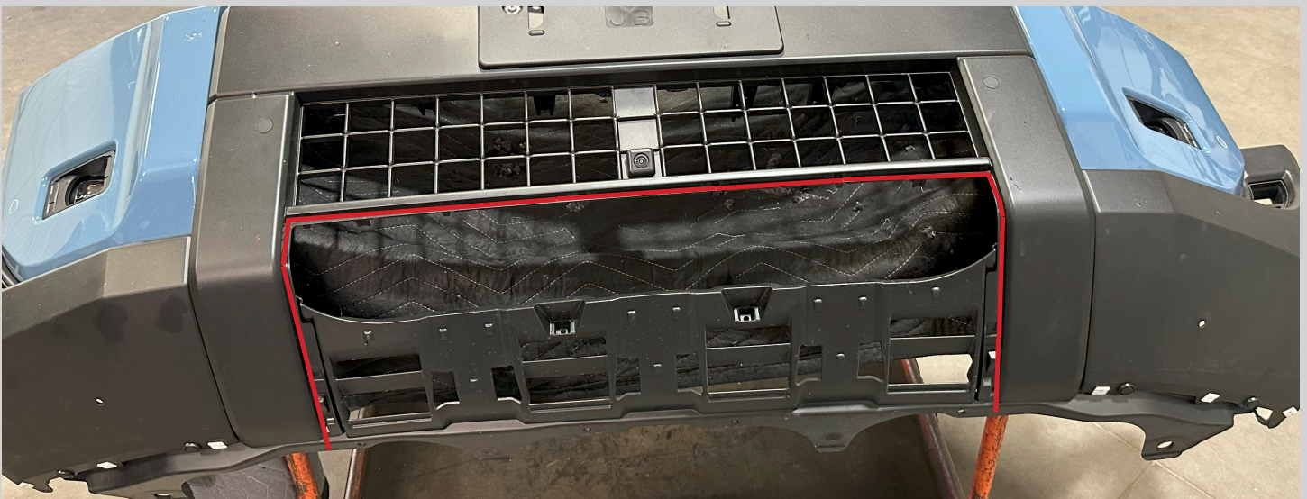
Figure 17: Cutline on the bumper cover.
