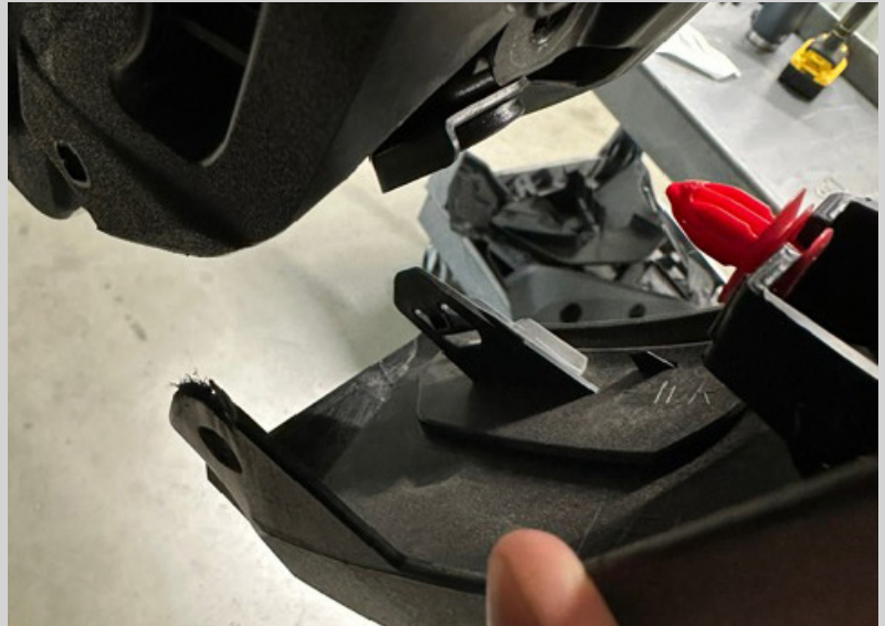
Figure 7: Clip on the fender flare.
