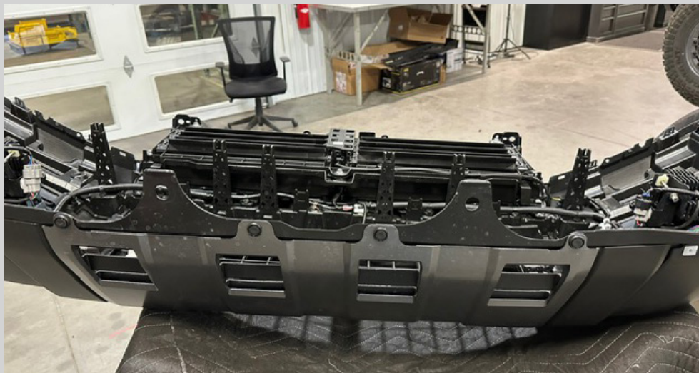
Figure 14: Remove the 4 plastic clips along the bottom edge.
