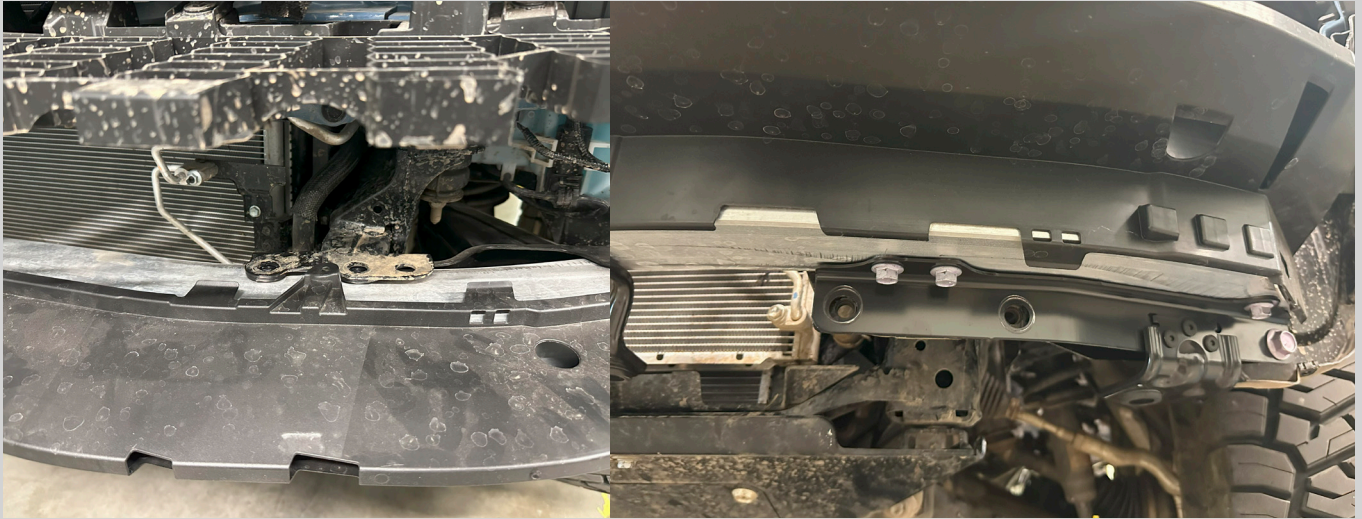
Figure 20: Remove the 8 bolts securing the crash bar and remove it.
