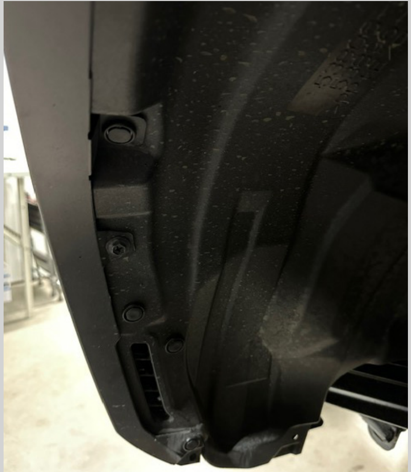
Figure 3: Clips and screws to remove along the front of the fender flares.
