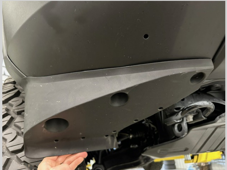
Figure 4: Lower air deflector to remove.
