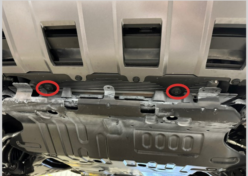
Figure 6: 2 lower bolts (10mm) to remove.
