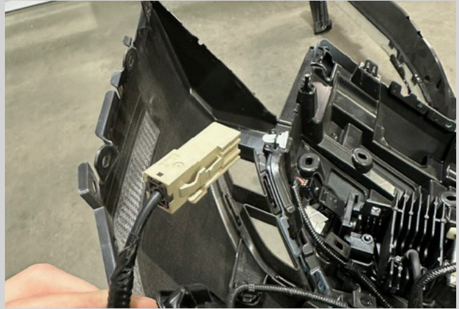
Figure 10: Plug behind driver side fender liner
