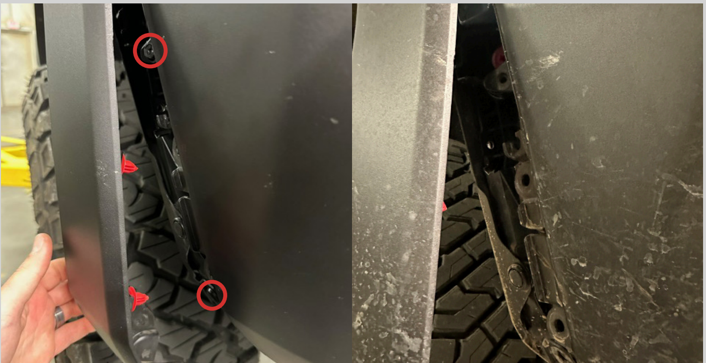
Figure 8: Left photo shows the screw (top of photo) and the clip to remove. Right photo shows the clip and screw removed.
