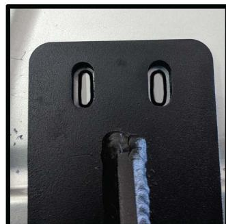
Install the front plusnut on each side of the vehicle and lightly bolt in the roof rack. Visually inspect the fit. Once satisfied mark the remaining slots to be drilled
