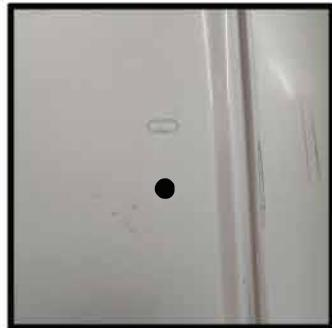
Work your way up to a 3/8" bit and then try to insert the plusnut. The recommended hole size from plusnut is .386"- .391"
