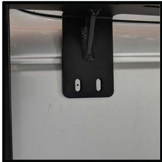
Place the roof rack on top of your vehicle aligning the front slots over your measured marks. If the rack looks well positioned you can now move on to drilling
