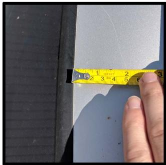
Measure back from the seam of the windshield as shown to a distance of  $9\frac{1}{4}$ " and mark on the driver and passenger side
